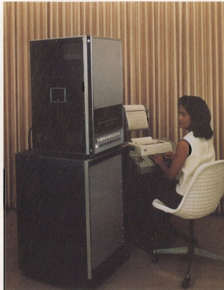
HP entered the computer market in 1966 with the introduction of the HP 2116A—basically a controller for instruments.
